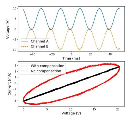
FIG. 7. Top: Shown are the voltage inputs into amplifiers A and B in Fig. 3 when the driving signal at C is a 10 V amplitude sine wave with a +10 V offset. Bottom: The I-V curve for a 3.3 k $\Omega$  resistor in place of the Langmuir probe with and without a compensating capacitance.
