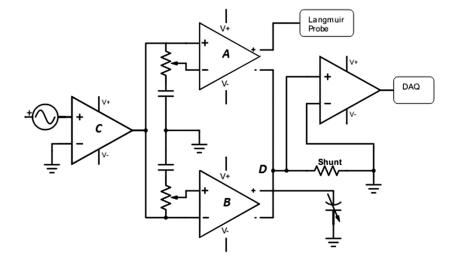
FIG. 1. Electronic schematic of the main components of the fast sweep probe system. Point D is where reactive currents undergo analog subtraction due to their inverted input voltage signals and the remaining plasma current is measured across the shunt using a low noise amplifier in parallel.
