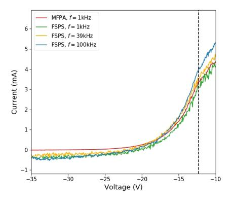
FIG. 8. I-V traces corresponding to the EEPFs in Fig. 3 during the validation experiment for different probe systems and sweeping frequencies. Dashed vertical line is located at the plasma potential.
