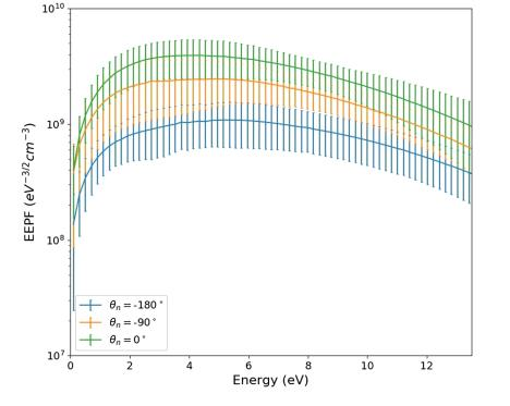
FIG. 6. Representative EEPFs at different phases of the spoke density oscillation. EEPFs are restricted below  $3T_e \approx 13.5$  eV.
