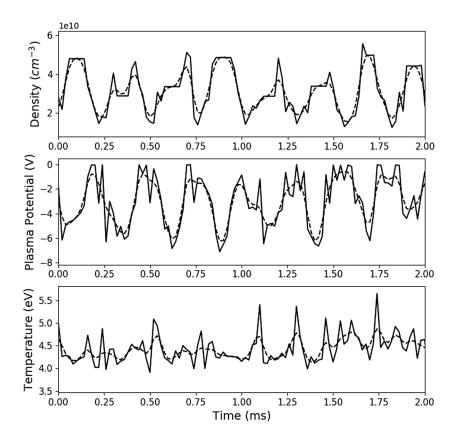
FIG. 4. A sample 2 ms time series of FSPS measurements. Each point is one voltage sweep. The underlying dashed curve is the result of a 2nd order low-pass Bessel filter at a cut-off frequency of 10 kHz.
